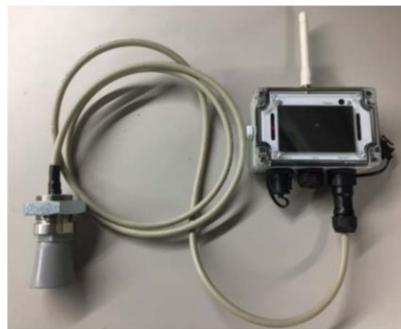
Figure 3:EnOcean self-powered sensor module with attached generic ultrasonic sensor
